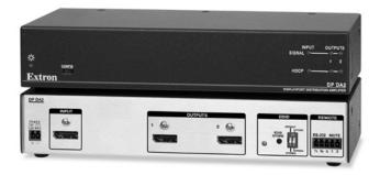
The Extron DP DA2 is a one input, two output DisplayPort distribution amplifier. It features EDID Minder® and Key Minder®, two Extron-exclusive technologies that automatically manage EDID communication and HDCP negotiation for reliable operation in commercial AV applications. The DP DA2 is ideal for applications that require the distribution of a DisplayPort source signal to two displays.
